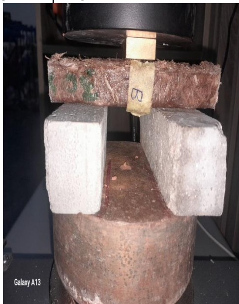
Fig 13; Sample placed on universal testing machine.
