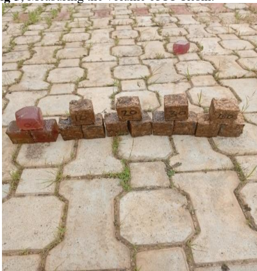
Fig 7; FRP composites at different volume factions For compressive, impact, density and water absorption test
