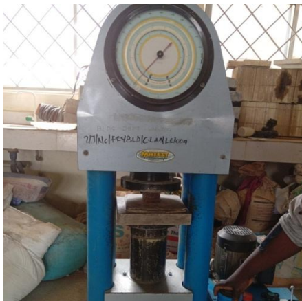
Fig 11: Universal testing machine testing the Compressive strength of the kenaf FRP composites
