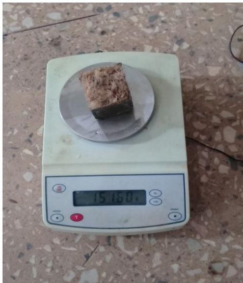
Fig 16; Measurement of kenaf FRP composites for density determination
