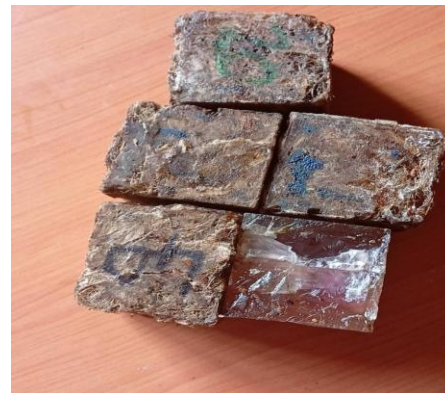
Fig 12: Crushed kenaf FRP composites
