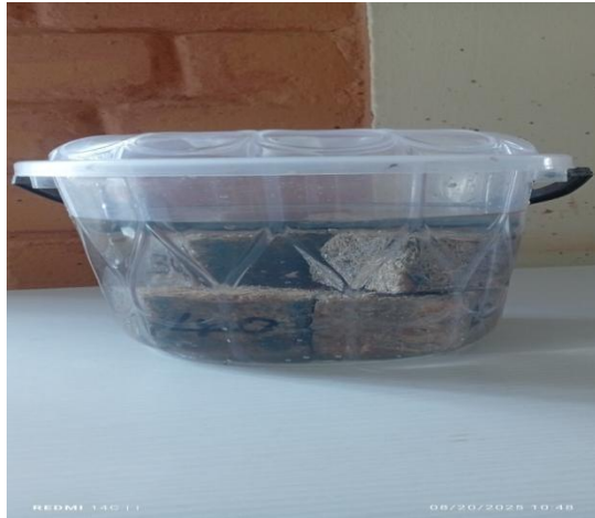
Fig 17; water absorption test of the kenaf FRP composites
