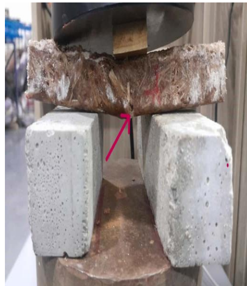
Fig 14; Break sample specimen after force applied
