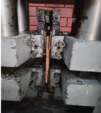
Fig 9; Sample on universal testing machine for tensile strength test
