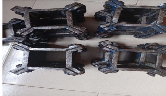
Fig 4; Iron fabricated mould
