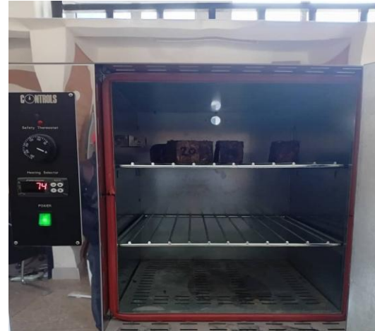
Fig 18; Heating of wet FRP composite at 105°C in oven.
