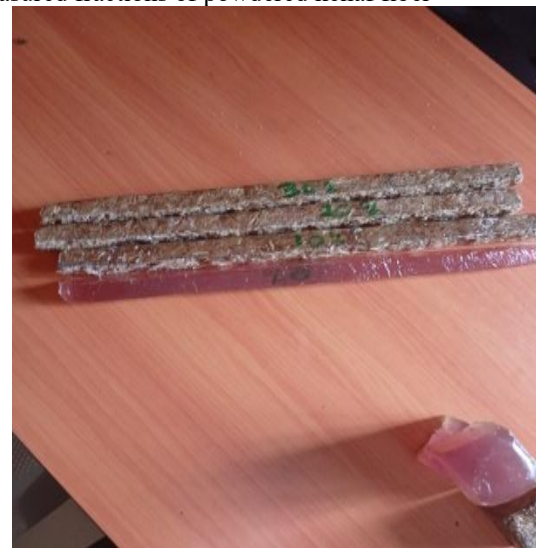
Fig 8; FRP composites at different volume factions for tensile strength and flexural strength test
