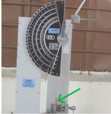
Fig 15; Sample specimen on Izod charpy impact testing machine.
