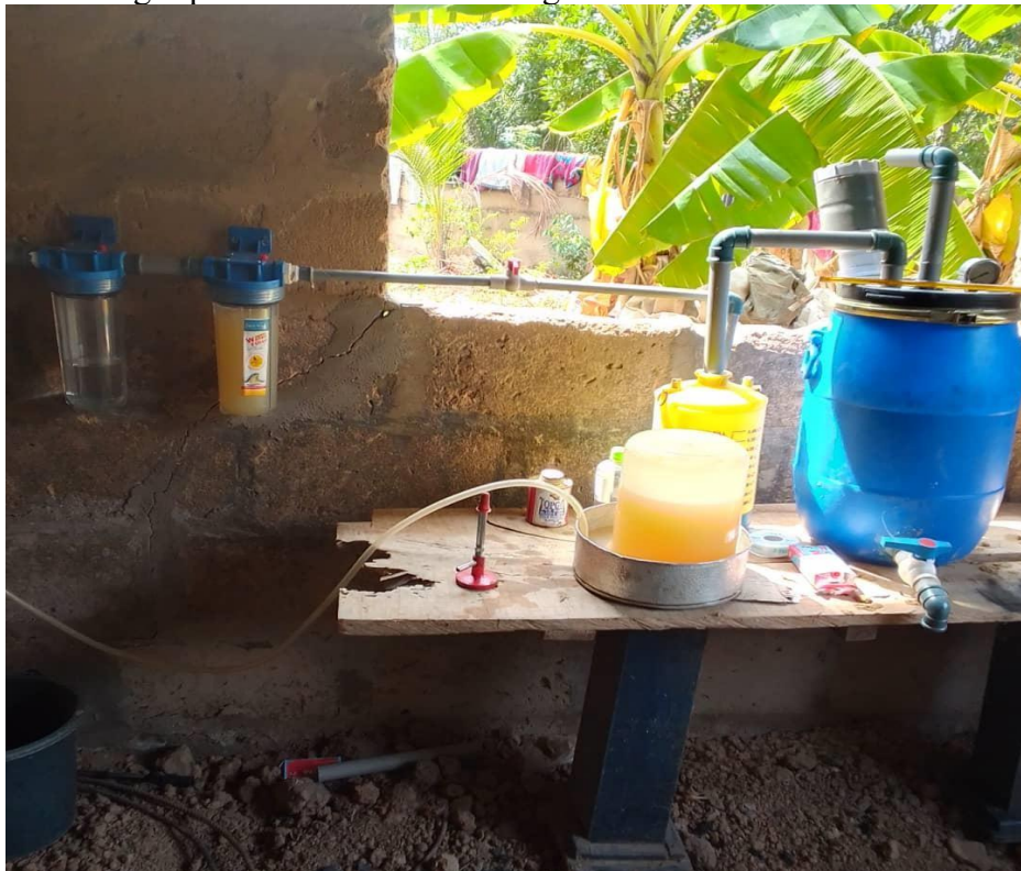
Figure8: Picture of the constructed plastic digester (By the Researcher)
